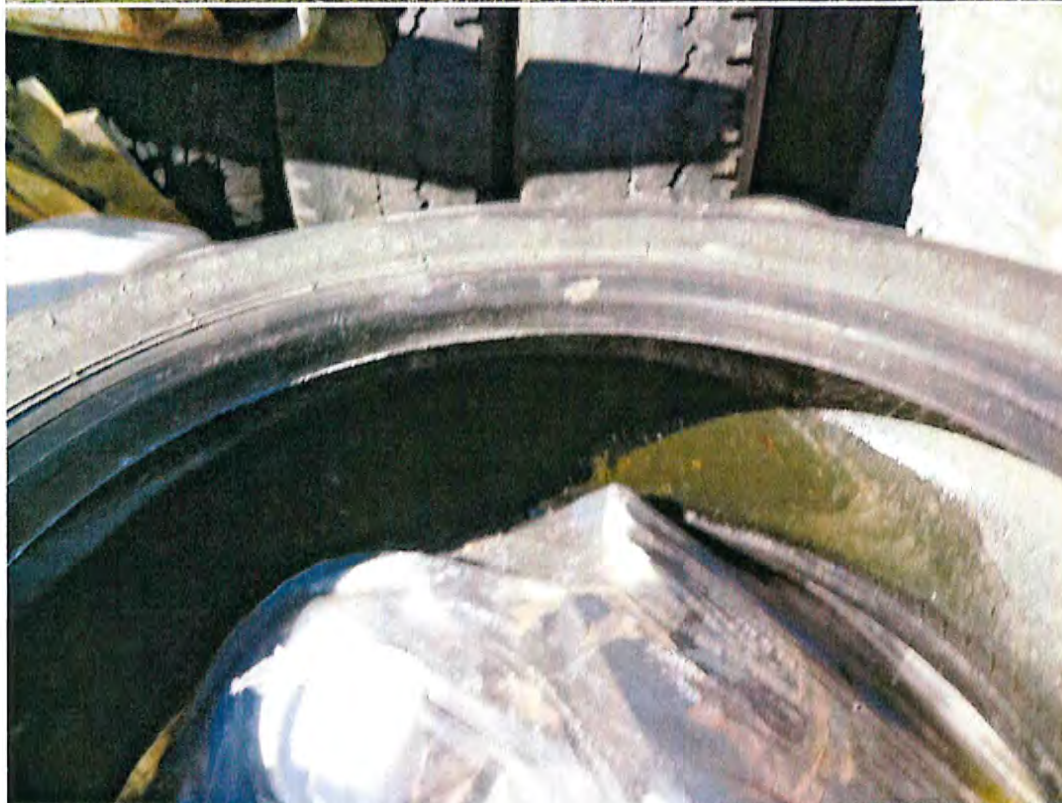
Date: 06/28/2013 Time: 9:01 a.m. Direction: down Photo by: Bill Gonet Exposure #: 010 Comments: Water in tire.
